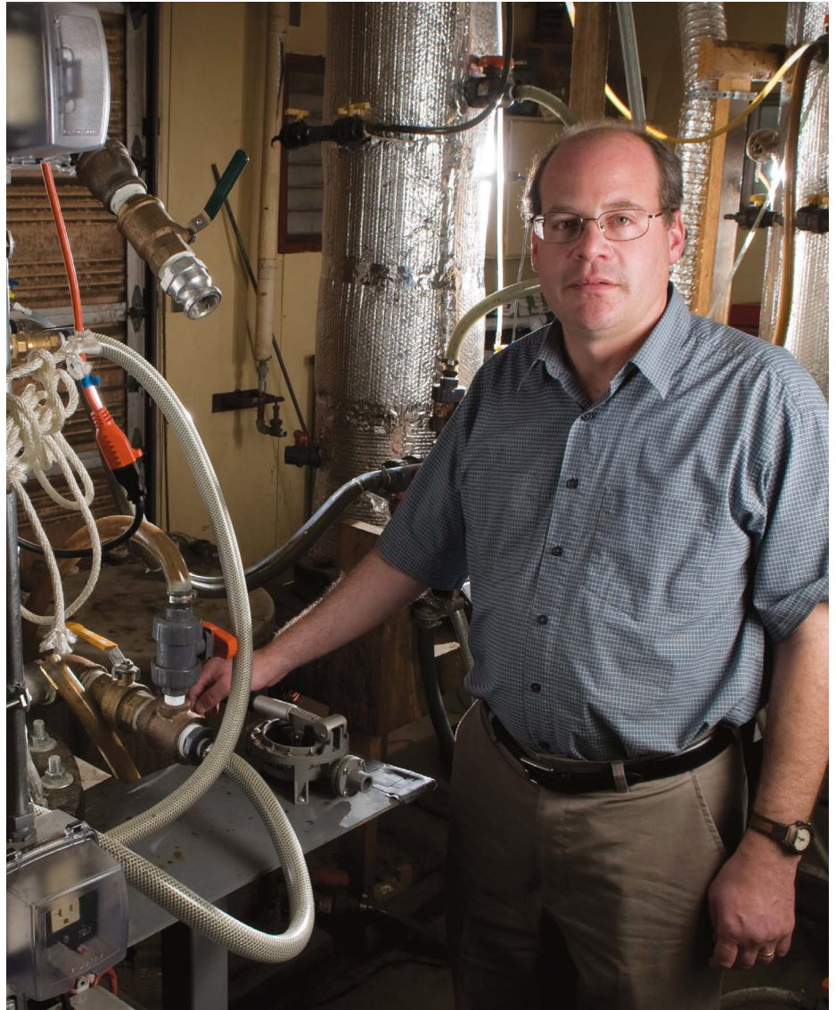
Steve Safferman with an anaerobic digester, a unit that uses microbiology to boost the energy producing potential of wastewater biosolids.
